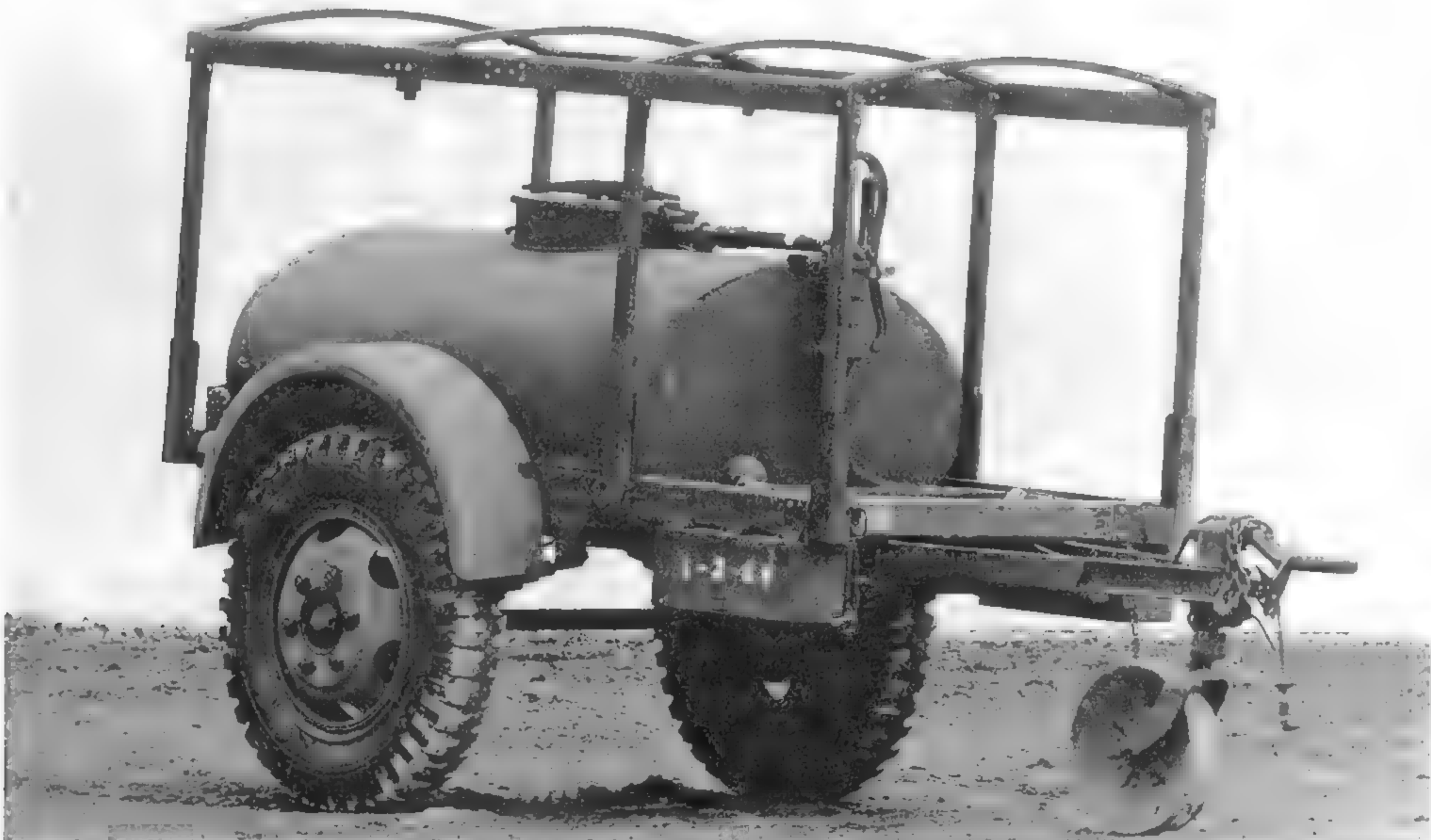
This Ben-Hur-built water tanker has the supports in place for a tarpaulin, which acts as camouflage to disguise this as a cargo trailer. Any specialized equipment, be it trucks or trailers, seemed to draw an unusual amount of enemy fire, so efforts were made to create a uniform appearance with normal cargo-carrying vehicles. The hand-operated dispensing pump can be seen mounted on the front of the tank. (U.S. Army photo)
